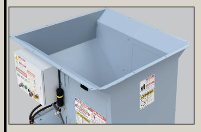
Hopper flange allows for bolt on deflectors and chute extensions when needed.
