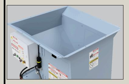
Hopper flange allows for bolt on deflectors and chute extensions when needed.
