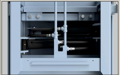
Innovative removable slider plate stops in combination with the removable carrier plates allow for slider plate to easily be pulled forward or completely removed.
