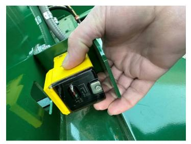
With the hopper empty, realign the eye by using the lights on the end of the photo eye. The green light should be the only one on when properly aligned. Rotate the photo eye up and down while watching the lights to find the best alignment. Tighten the black nut by hand. Do not over tighten.
