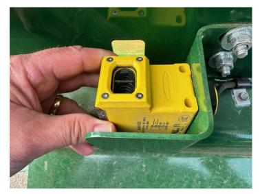
Cleaning the photo eye is a normal task in maintaining an apartment style compactor. The standard photo eye on our PX50 does not use a reflector. To clean it simply loosen the black nut and turn the photo eye face up. Clean the eye with a damp cloth. DO NOT use harsh chemicals or brake clean. If needed, use a glass cleaner.
